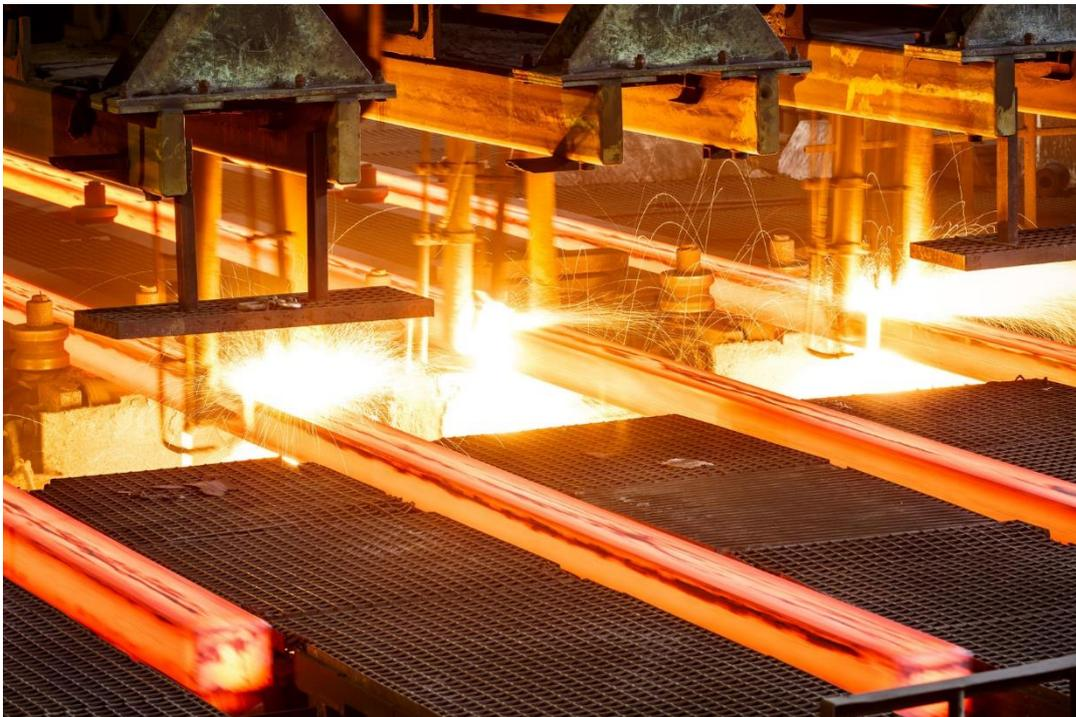
Red-hot steel billets on their way to be processed. Source: zhaojiankangphoto via 123RF.com.
